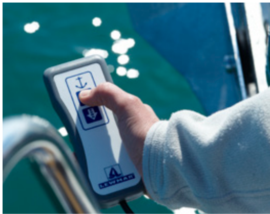
Anchor windlass, electrical with remote control
