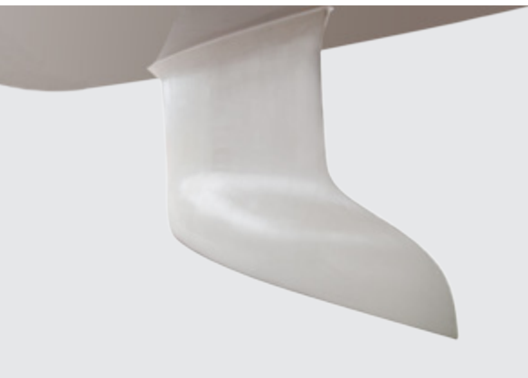
Shallow draft L-shaped keel, cast iron, 1.55 m draft
